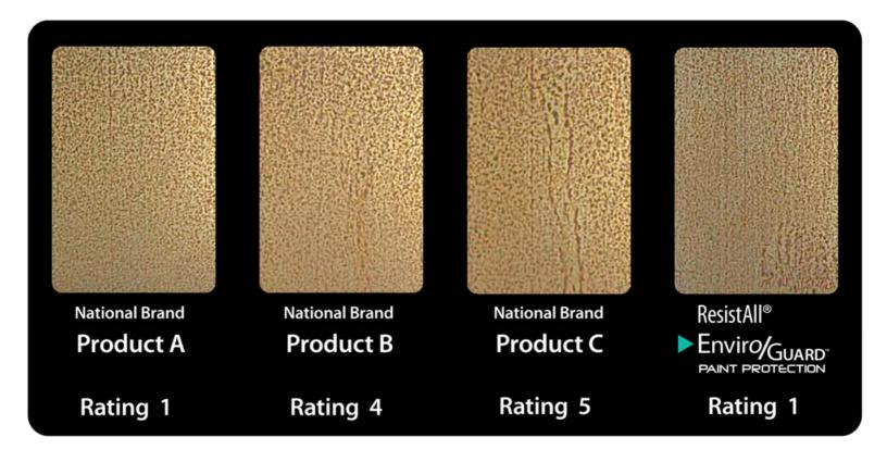
Figure 8: Samples after 70 minutes salt spray exposure.
