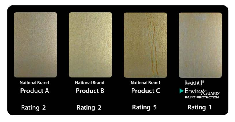
Figure 3: Samples after 20 minutes salt spray exposure.
