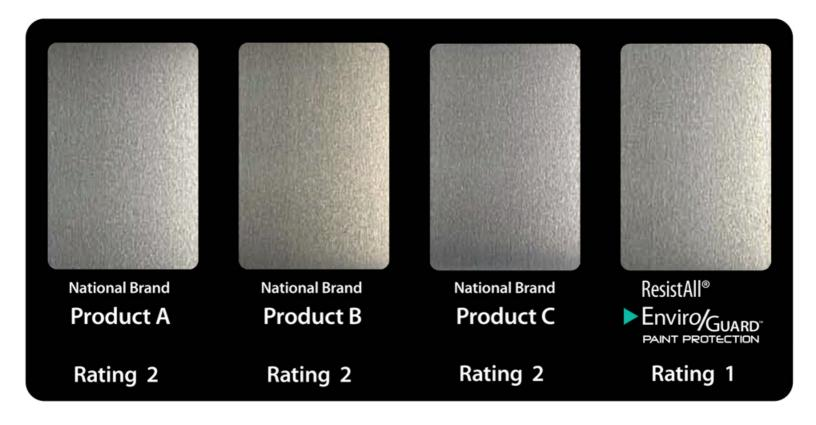
Figure 2: Samples after 10 minutes salt spray exposure.
