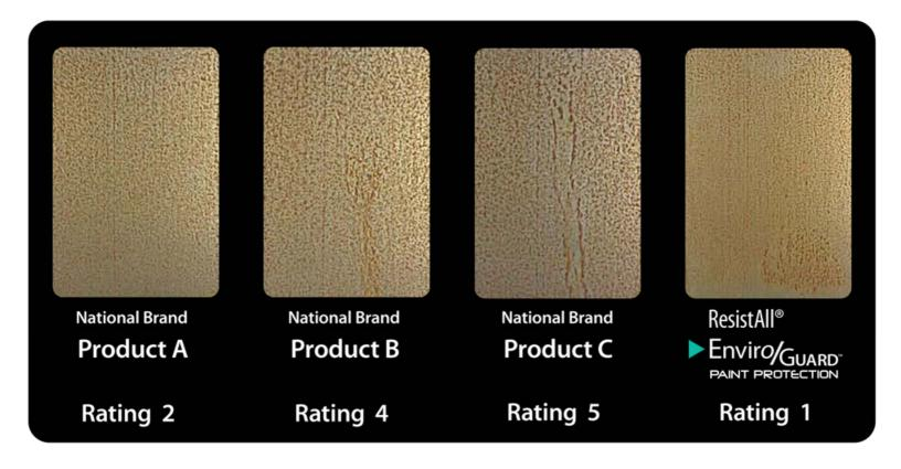
Figure 6: Samples after 50 minutes salt spray exposure.
