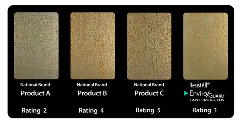
Figure 5: Samples after 40 minutes salt spray exposure.
